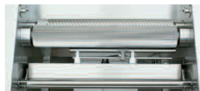
NOCK Air Jet compressed air cleaning system: Jet bar moved by an enclosed pneumatic cylinder
